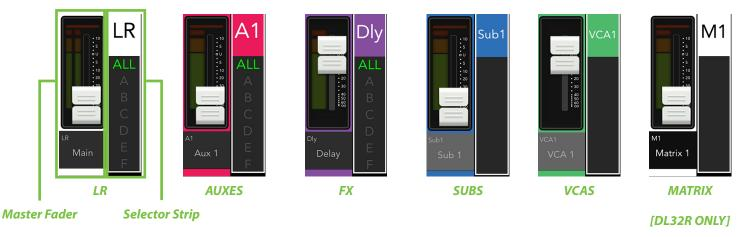
**Selector Strip** – Top to bottom, the selector strips breaks down to two separate selectors:
