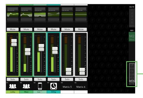
• **Step 5** — Remember when we set up talkback to the matrix outputs back in step 1? Tap the quick access panel, tap the talkback button and make your very important announcements (making sure the talkback level is set appropriately).
