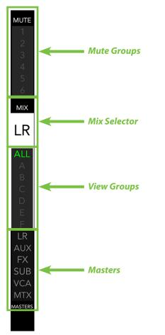
Top to bottom, the selector strip breaks down to four separate selectors:
