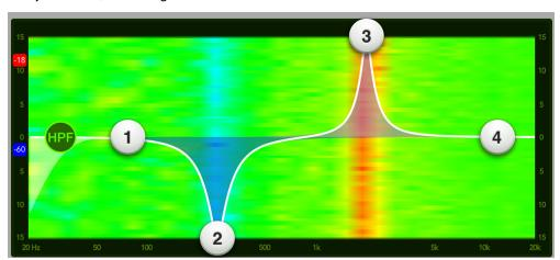
• Band 3 has a +15 db boost at 2 kHz which may be seen on the spectrograph as a narrow red and yellow line, indicating that the level has been boosted at 2 kHz.
