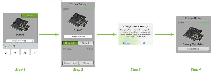
In addition to renaming the mixer, setting up the device also means that you may change the mixer's IP address. This begs the question why? Well, if the mixer is used in a complex network, such as a church or other fixed install, it allows the mixer to work better in that environment. This is because the mixer will remain at the same IP address, allowing IT to set up and better monitor the devices.
