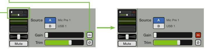
DL32R 48v Phantom Power Disengaged
