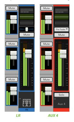
Navigate to the delay return channel, then move the channel fader up and down. Notice that it also moves the delay return fader up and down. This is because they are both showing the same level. As such, moving the return delay fader up and down also moves the delay channel fader up and down. This works with the reverb return channels and reverb return faders, as well.
