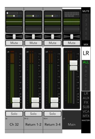
**48V / Gain** — By default, 48V and gain on the return channels is absent from the input routing view for these two channels. However, the source and trim will still be displayed and input routing may still be accessed in order to update channel and aux send assignments.
