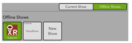
At this point the show has been created, but it is still an Offline Show. It has to be the Current Show in order to view and load snapshots. That's easy! Just tap the Headliner button to reveal a popover similar to what is displayed at the top of this page. From there tap the red Load button to reveal an image similar to what may be seen below.
