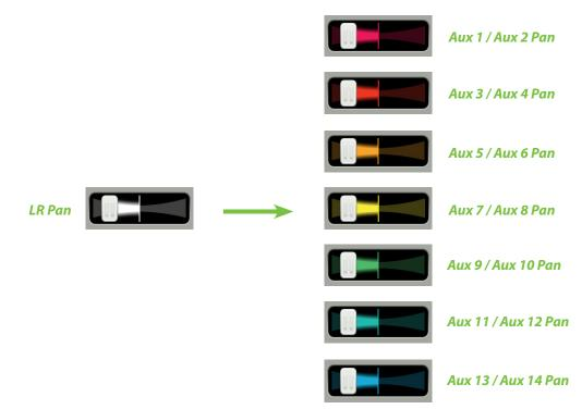
For a linked aux, the user may de-select Use LR Pan (on the iPad) to control the aux pans and main mix pans independently for each channel. An example of this is displayed below.
