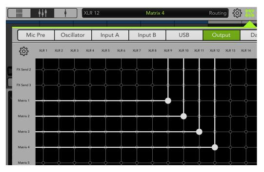
There IS one additional thing we can set up while the I/O patch is still open: talkback. Tap the talkback tab and swipe left. Assign talkback to matrix 1-4.
