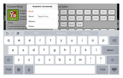
Tap inside of the blank "Name:" box to reveal the onscreen keyboard, then name the currently selected snapshot as you so desire. Tap the "return" key when satisfied with the name. If the name is too long to fit, the button scrolls, displaying the entire name.
