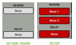
**Mute Reverb(s) / Delay** — Tapping the reverb and/or delay mute button in the quick access panel is akin to tapping the LR mute button at the top of the reverb and/or delay channel strip. However, with the quick access panel, you now have easier access to the effects controls regardless of what view is open.
