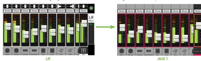
**Channel ID Button** – Each channel ID button name and image is user-editable. Additionally, users may also link two adjoining channels together into a single channel strip. Simply tap the button at the very bottom of the channel strip to reveal a popover that allows editing of the name, image and color and an option to link channels.
