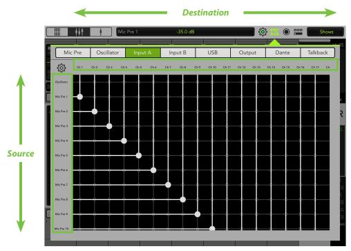
The source and destination may change, but the default patching for each channel input A is mic pres 1-32 routed to channels 1-32 and USB 1-4 routed to returns 1-4. Additionally, mic pre 32 is routed to talkback. Drag anywhere in the black box to view these other routings.
