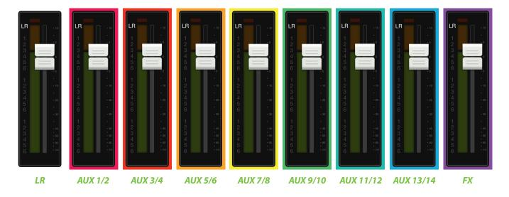
All we did was change the selected output from main LR to aux 1. Notice below how each channel's input meter is surrounded by the color of the selected output. In the left image, the faders control the levels going to the LR mix, while the faders on the right image control the levels going to the aux 1 mix.
