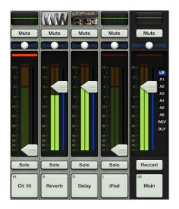
• Fast access to dynamics — Tapping the gain reduction meter takes you straight to the dynamics view.
