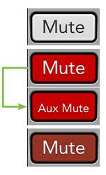
**Mute** – Mute buttons do just what they sound like they do. They mute – turn off – the signal on the channel(s). Engaging a channel's mute switch provides the same results as sliding the channel fader all the way down.
