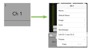
Each channel ID button name, image, color and preset is user-editable. Additionally, users may also quick assign the aforementioned, link two adjoining channels together into a single channel strip and/or copy the channel's characteristics in order to paste them to other input channels. To get started, simply tap the button at the very bottom of the channel strip to reveal a popover.
