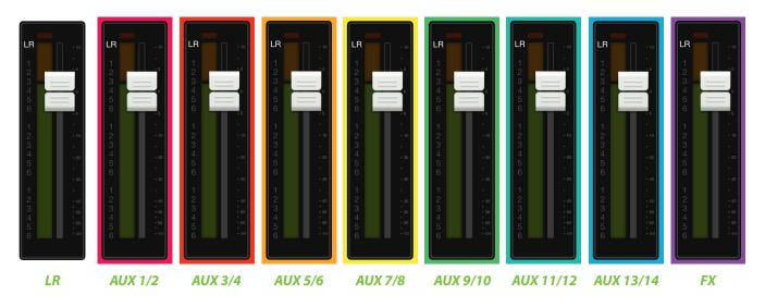
In the images below, all we did was change the selected output from LR to A1. Notice how each channel's input meter is surrounded by the color of the selected output.
