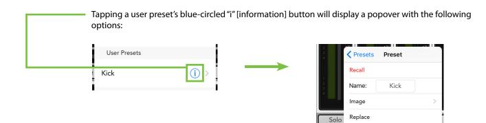
**Recall** — Pressing the recall button recalls presets. On recall, all appropriate console parameters change to match the stored preset. Recall is the only available option with factory presets. A confirmation dialog will appear.
