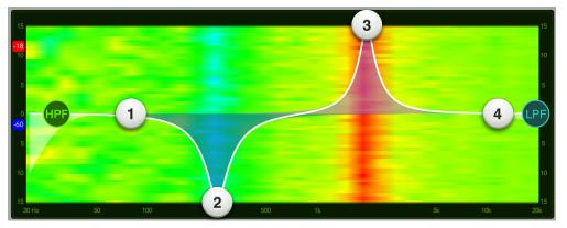
The RTA / spectrograph is available on all channel inputs and outputs. There is only one instance of the RTA implemented in the mixer. Therefore, only one channel can show the RTA or spectrograph at a time regardless of how many iPad devices are connected.
