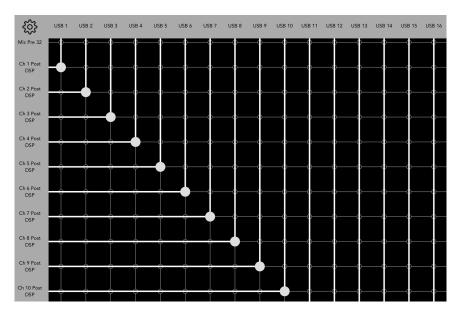
**OUTPUT 1** — Perhaps the DL32R will be used strictly as a monitor mixer with no need for main L/R. Here you're able to use all 14 outputs as linked aux sends for a total of seven in-ear and/or 14 wedge monitors.
