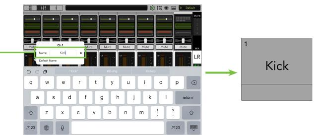
Before moving on with the rest of the Channel ID, let's look at another exciting feature regarding channel naming. On the left and right side of *Name:* are "previous" and "next" arrows<sup>2</sup>. This makes it easier to edit the names of multiple channels in a row without having to re-tap each channel's ID button just to name it.
