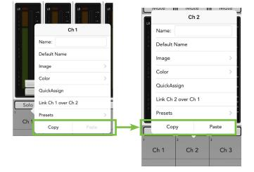
• Settings of an input channel to other input channels.
