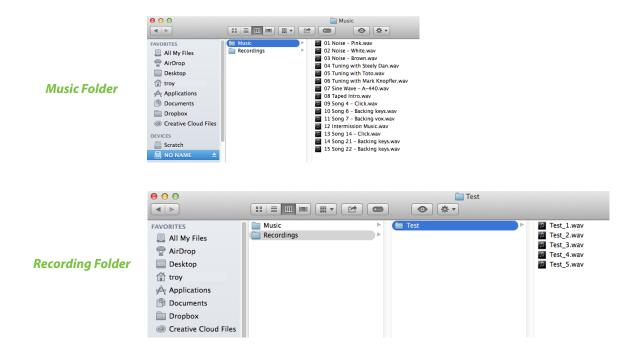
The recordings folder, on the other hand, is nothing but subfolders. Ok, ok, perhaps not in the example shown above. A subfolder is created for each recording. So after performing multiple recordings there would be multiple subfolders, each named with the name you provided. So, each subfolder contains a different recording made up of at least one .wav file. Longer recordings will yield more .wav files but we'll get to that in a second.
