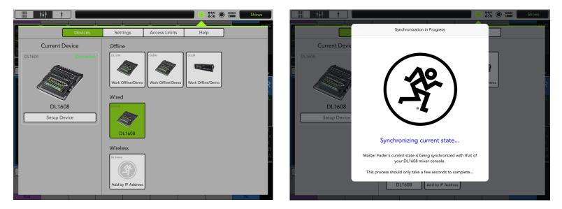
Switch between the offline and wired device selections and notice that the Master Fader app re-syncs with the console's current state every time you reconnect. The mixer is shown in full color in both devices [offline and wired] indicating that either may be selected. The router hasn't been set up yet, so there aren't any wireless options at this point.
