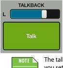
**Talkback** — The DL32R has a talkback level (L) and button. Channel 32 is the default for the talkback input. The talkback level slider controls the level of the talkback mic with the gain ranging from  $-\infty$  to +10 dB. Talkback may be routed to the main L/R, any subgroup, aux send and/or matrix. Refer to the I/O patch on pages 184-196 for more information.
