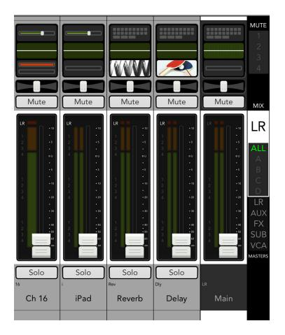
**No Digital Trim** — There is no digital trim on FX channels, so it will be absent from the input routing view for these two channels. However, input routing may still be accessed in order to update channel and aux send assignments.
