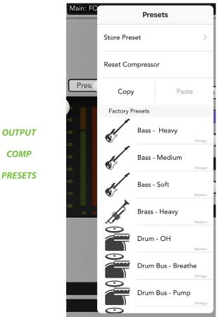
And from the compressor / limiter channel view you are able to set a preset for the compressor / limiter. Don't forget to scroll up to access more factory presets, if going that route. These presets recall the compressor / limiter type [modern or vintage].
