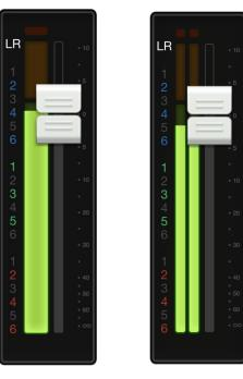
The touch sensitive faders adjust the level of each channel going to the selected output. Adjustments are made by touching and dragging channel faders up and down. Touched channel faders will "grow & glow" to indicate that they are being adjusted. The fader level ranges from  $-\infty$  to +10 dB as indicated by the scale on the right.
