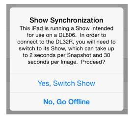
**Yes, Switch Show** – tapping this button will change the current show on the iPad to match the same show as is currently on the mixer. It will take about two seconds per snapshot to synchronize the shows. All connected iOS devices will automatically sync with the current show.
