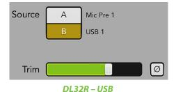
If a source without a mic pre is selected – USB 1 (above right, for example) – the gain and 48v controls are hidden.
