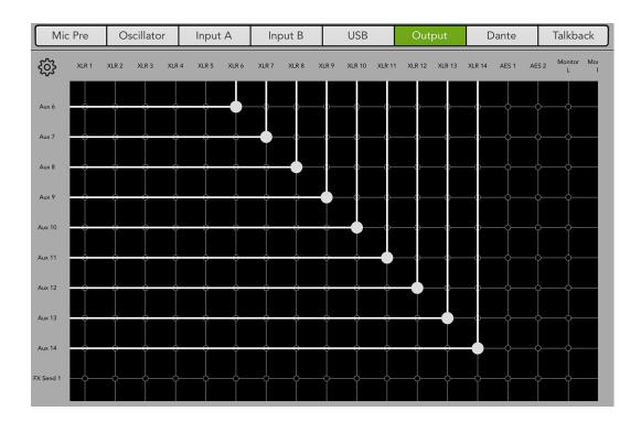
**OUTPUT 2** — Another output patching example might be found in a typical theatre setup. Here, the main L/R would be the PA and all six matrix outputs will be dialed in, as well, sending signal to the theatre's lobby, mezzanine, bathrooms, etc. (all with unique settings).
