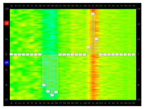
The RTA / spectrograph is available on all channel inputs and outputs. There is only one instance of the RTA implemented in the mixer. Therefore, only one channel can show the RTA or spectrograph at a time regardless of how many iPad devices are connected.
