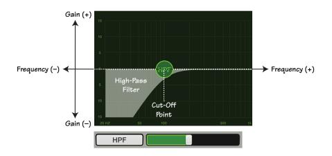
High-Pass Filter (Disengaged)
