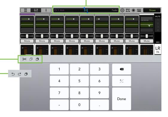
Also, if you want to type in an exact value for a parameter, touch the channel's parameter you would like to update so it appears in the current parameter display. Next, tap the current parameter display; a numeric keypad appears. Simply type in the exact value you would like for that channel's parameter followed by tapping the "Done" button.
